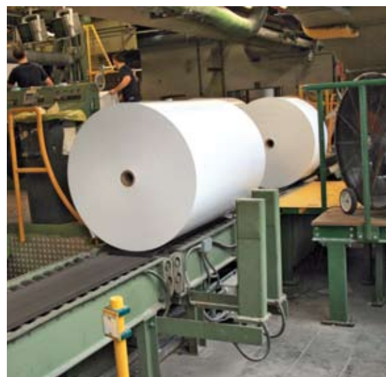
Siegling Transtex can easily handle punctual loads of 1500 kg without damaging the layers of paper on the outside.
