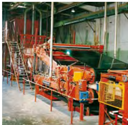
Pre-press belt in the manufacture of particle boards. The particle mat is pre-pressed while being conveyed.
