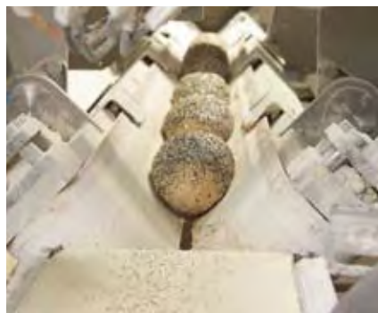
In large bakeries balls of dough are formed as a result of differing belt speeds.
